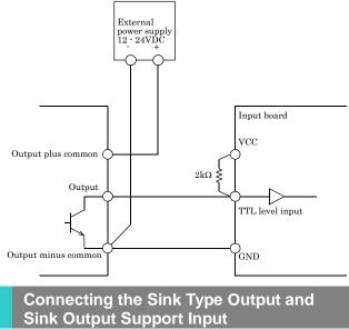
The following example shows a connection between a sink type output (output board) and a sink output support input (input board). Refer to this connection example when you connect such boards to each other.
