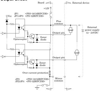
The output circuits of interface blocks of the PIO-16/16B(PCI)H and this product are illustrated the image
